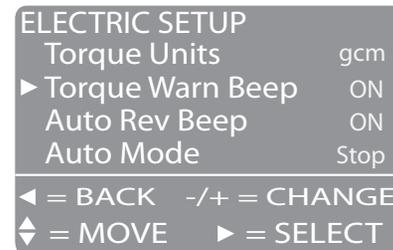
5. Specify other electric handpiece options by pressing minus (-), plus (+), and ► to move through the screens. Once the setup is complete, three beeps confirm the setting for all handpieces.
